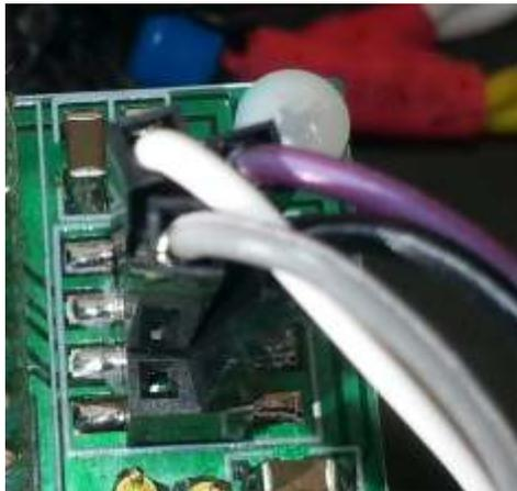
Figure 3: RPi B or RPi-DAC I2S (P5)
